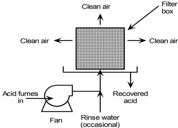
**Sulfuric acid fume filter system**
