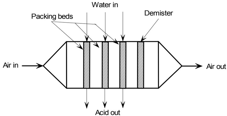
**Components of a multi-stage crossflow scrubber**
